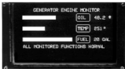
The APD-192G088 is a full field dot matrix display with 192 columns and 88 rows. It includes drive electronics and a microprocessor based controller. The controller maintains all the refresh memory, character generation and control logic with parallel or serial interface and a DC to DC converter to generate the necessary panel voltage. A touch panel version is also available (APD-192G088-5).
