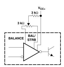
NOTE: If offset balancing is not used, the BALANCE and BAL/STRB pins should be shorted together.
