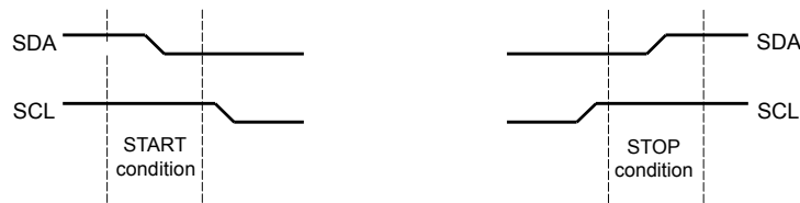
Figure 15-3. START and STOP Conditions
