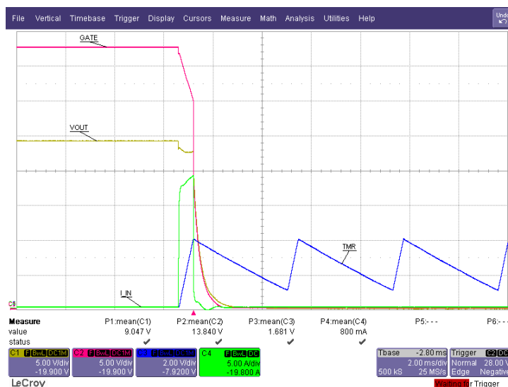
Figure 34. TPS2483 Retry-Cycle Timing Detail
