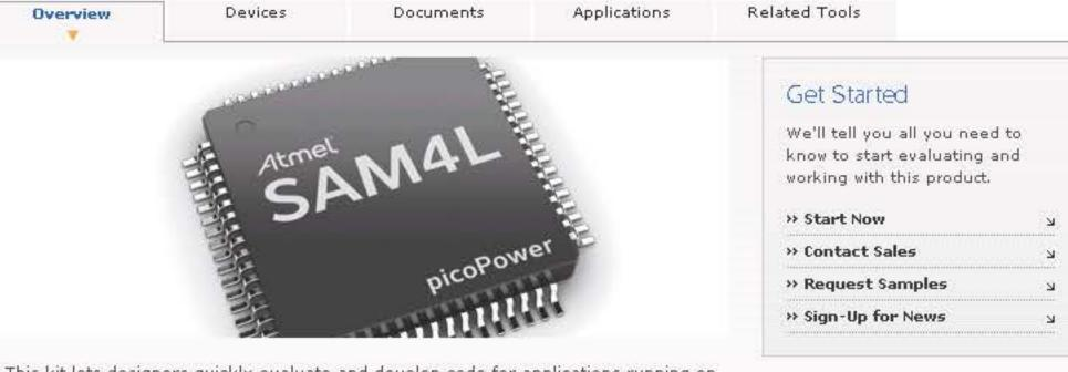
This kit lets designers quickly evaluate and develop code for applications running on Atmel SAM4L microcontrollers. The board features an embedded debugger, dedicated circuitry to measure the power consumption of your application, LCD, USB, capacitive touch functionality and much more. It also offers expansion headers to plug in Atmel extension boards so you can easily add gyrometers, accelerometers, Wifi and Zigbee to your SAM4L-EK.
