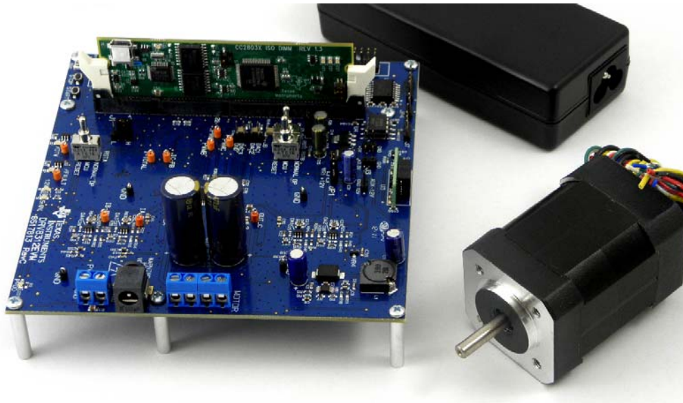
Figure 1. DK-LM3S-DRV8312 Kit (Stellaris® Version)
