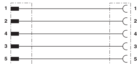
Contact assignment of the M12 connector and the M12 socket
