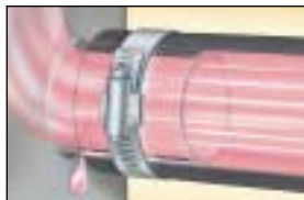
Non-compensating clamp cannot adjust during extreme temperature changes, allowing leaks to occur
