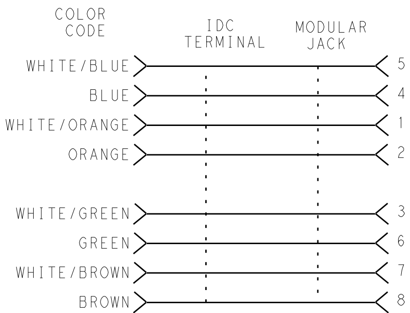
ELECTRICAL SCHEMATIC T568B
