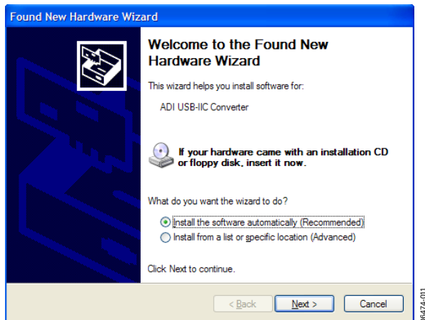
Figure 11. Automatically Installing Drivers for the Evaluation Board
