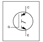
600 V  $I_{C(nom)} = 35\text{A}$   $V_{CE(on)} \text{ typ.} = 1.6\text{V} @$   $I_{C(nom)} @ 25^{\circ}\text{C}$ Motor Control IGBT
