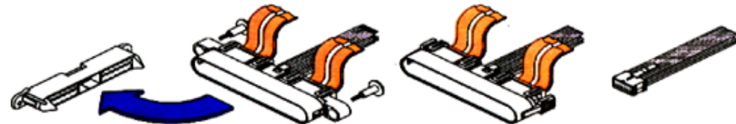
4, 6, OR 8 POWER CIRCUITS & 21 SIGNAL CIRCUITS
