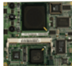
ETX CPU Module with AMD® LX800 CPU on-board, USB 2.0, LAN & Audio
