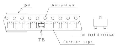
Those with one electrode terminal on the feed hole side·····TB
