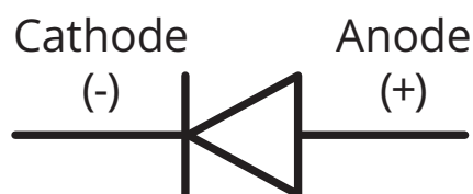
Figure 1b. Polarity of L1SP-PRPxx03500000, L1SP-RYL0003500000 and L1SP-LME0003500000.
