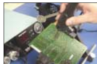
The DSV80 80-watt desoldering tool is perfect for desoldering through-hole components.
