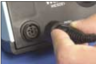
The new connector and plug on the WES51 is an improvement over the WES50
