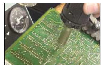
Through hole rework with the DSV80
