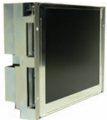
6.4" open frame display, high bright, sunlight readable with heater and video interface for outdoor banking application
