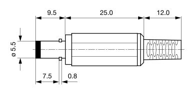
Cable diameter max. 4.0 mm
