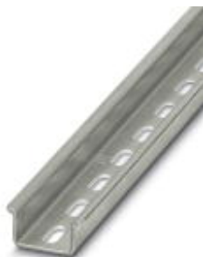
DIN rail perforated, Standard profile, width: 35 mm, height: 15 mm, similar to EN 60715: 2001, material: Steel, uncoated, length: 2000 mm, color: white aluminum
