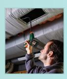
Extech Borescope features a 2.4" color monitor with video output for viewing on any monitor and a waterproof 9mm camera with bright LED lights.
