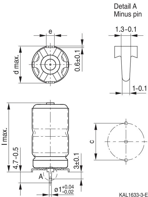
Mounting holes d = 16 mm ... 21 mm
