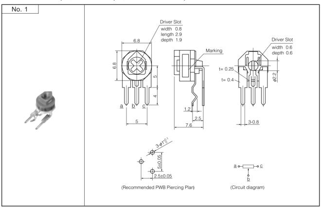
• 3-terminal, Top-adjust, Both Sides Adjust, Cross Slot Screw Adjust...... EVM4LG
