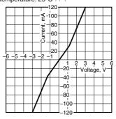
9. Off state leakage current vs. load voltage characteristics
