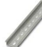
DIN rail, material: steel galvanized and passivated with a thick layer, perforated, height 7.5 mm, width 35 mm, length: 2000 mm
