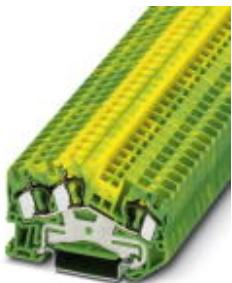
Feed-through terminal block, Connection method: Spring-cage connection, Cross section: 0.08 mm<sup>2</sup> - 6 mm<sup>2</sup>, AWG: 28 - 10, Width: 6.2 mm, Color: green-yellow, Mounting type: NS 35/7,5, NS 35/15
