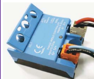
Pluggable removable input spring connectors Minimum: AWG28 Maximum: AWG14
