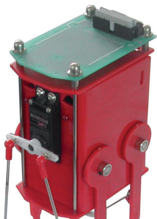
Installing experiment PCB
