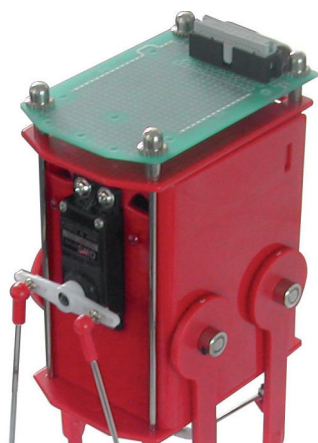
Installing experiment PCB
