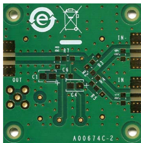
Figure 2. Circuit Side of Evaluation Board
