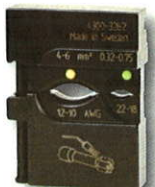
43162 PortaCrimp Die set for heat shrink connectors: 4-6mm 2 yellow & 0.32-0.75mm 2 green.
