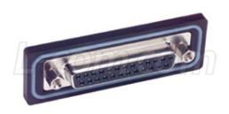
Networking and Other Equipment Harsh outdoor or indoor environments can destroy electronic equipment. Standard D-sub connectors are not intended to withstand contaminants such as water and dust. This waterproof solder cup DB25 female connectors will accommodate wire ranges from 30 - 20 AWG. Construction features gold plated brass contacts, nickel plated steel shells, and a silicone insulating ring. Maximum recommended panel thickness is 0.078"
