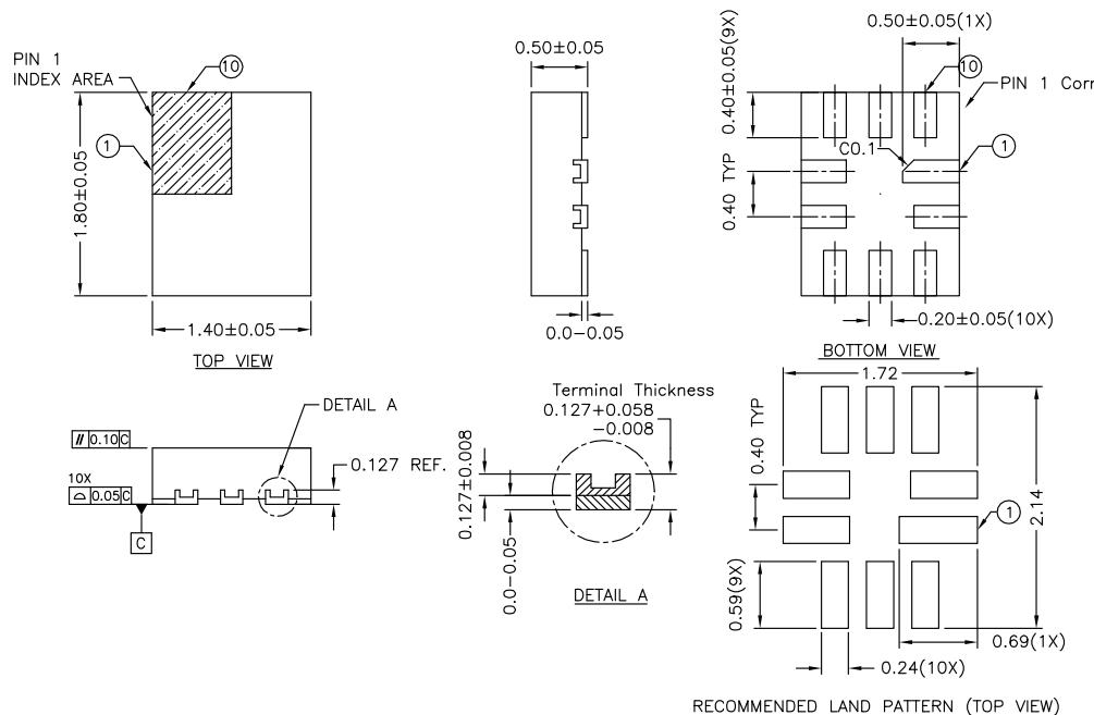
**Package Mechanical: 10-Contact, TQFN (ZL)**
