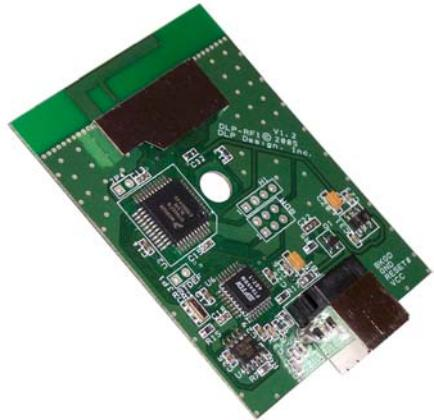
The MC9S08GT60 can be reprogrammed (if desired) with user-supplied firmware via a 6-pin BDM header that is compatible with the P&E USB-ML-12 and other device programmers (purchased separately).
