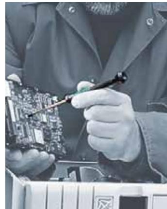
The fixed head and the fast-turning zone just below the head allow **rapid twisting**. This makes time-consuming grip adjustments, as required with other conventional precision screwdrivers, unnecessary.
