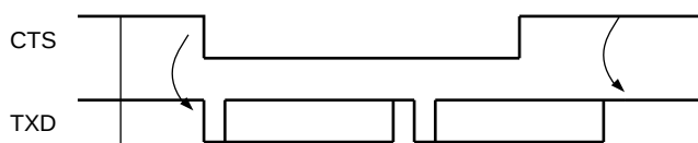
Figure 39-28. Transmitter Behavior when Operating with Hardware Handshaking
