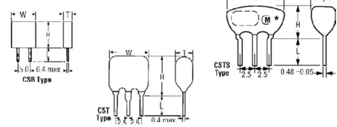
Features of ceramic resonators include low cost, good stability, small size and rugged construction, and a wide frequency range. Specifications. Frequency Range: CSB Type — 375 to 1250 KHz; CST Type — 1.80 to 70 MHz; CSTS Type — 3.4 to 10 MHz. Frequency Tolerance: ±0.5%. Temperature Stability (-20°C to +80°C): CSB and CST Type — ±0.3%; CSTS Type — ±0.2%. Time Stability (10 Years): CSB and CST Type — ±0.3%; CSTS Type — ±0.2%.
