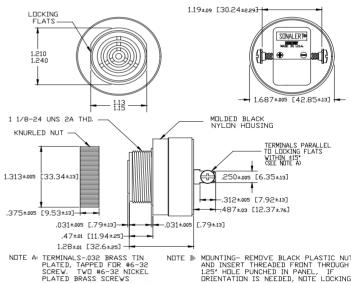
NOTE A: TERMINALS-0.02 BRASS TIN PLATED, TAPPED FOR #6-32 SCREW, TWD #6-32 NICKEL PLATED BRASS SCREWS INCLUDED, WILL ACCEPT 1/4' QUICK CONNECT.
