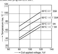
2. Ambient temperature characteristics and coil applied voltage
