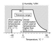
\* -40 to +85°C -40 to +185°F (When 45% to 80%V of coil holding voltage)
