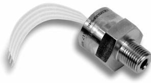
Honeywell's 13 mm Series stainless steel pressure sensors are designed for high pressure applications that involve measurement of hostile media in harsh environments. This series uses Honeywell's proven piezoresistive semiconductor sensor chip in an oil-isolated housing with or without an integral ceramic for temperature compensation and calibration. This design has proven to be highly reliable, stable and accurate.
