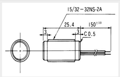
Case material: Glass filled Nylon 6 Wire: UL-1007, AWG #20 Dimensions in mm (1 mm = 0.0394 inches)
