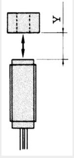
Magnet TG-0141 OFF (operate point): Y=5.5 mm ON (release point): Y=14 m
