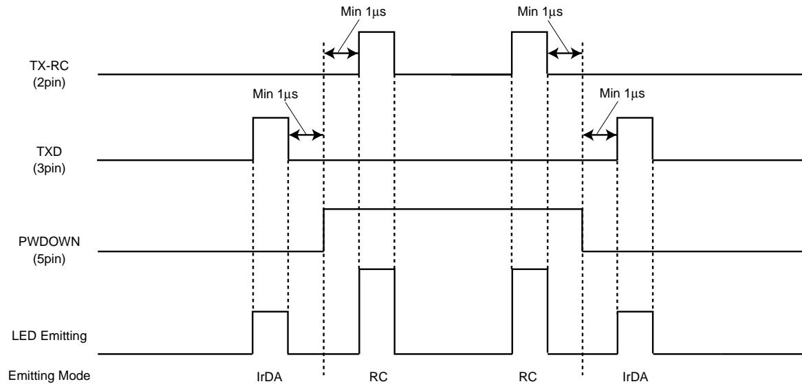
\*If TX-RC or TxD input pulse width is wider than 48μs, output LED emitting pulse will be turn off approximately 48μs.
