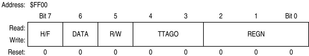
Figure 18-5. BDM Instruction Register (INSTRUCTION)
