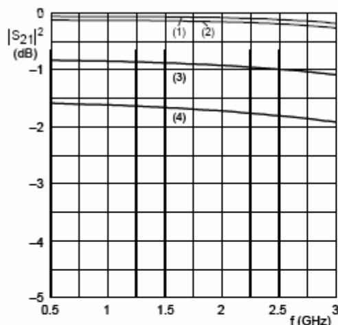
(1)  $I_F = 100 \text{ mA}$ . (3)  $I_F = 1 \text{ mA}$ .
