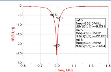
This antenna has about 20MHz of guardband on each side
