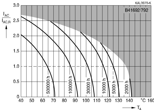
**Useful life<sup>1)</sup>**depending on case temperature  $T_C$  under ripple current operating conditions at  $V_R$
