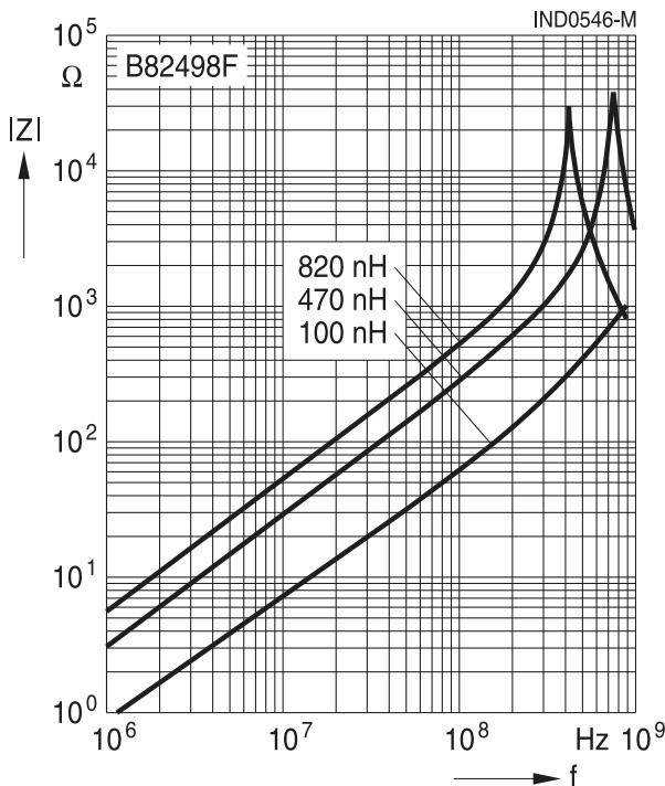
**Impedance  $|Z|$  vs. frequency  $f$  (ferrite core)**
