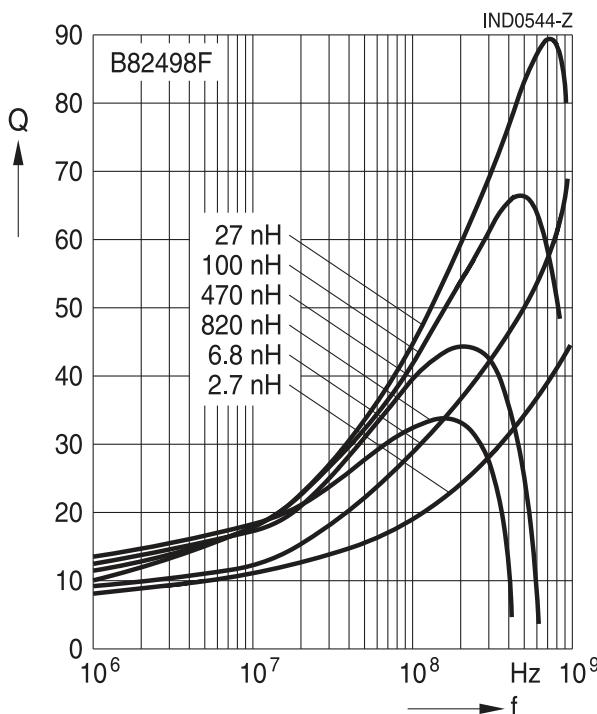
**Q factor versus frequency  $f$  (ferrite core)**
