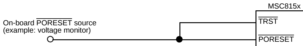
Figure 35. Reset Connection in Functional Application
