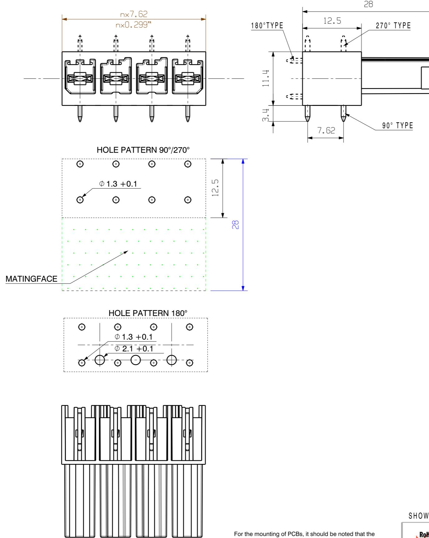
For the mounting of PCBs, it should be noted that the rated data given in the catalogue relates only to the connection elements. The necessary creepage and clearance paths must be observed in connection with the respective applicant in accordance to VDE 0110. The current-carrying capacity and pitch tolerance is to be determined according to DIN IEC 326 part 3 very fine.
