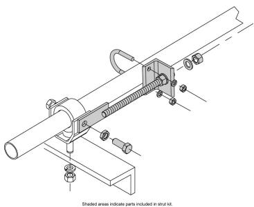
Azimuth Adjustment Kit
