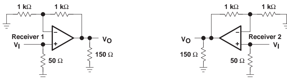
Figure 2. Receiver Input-to-Output Crosstalk Test Circuit
