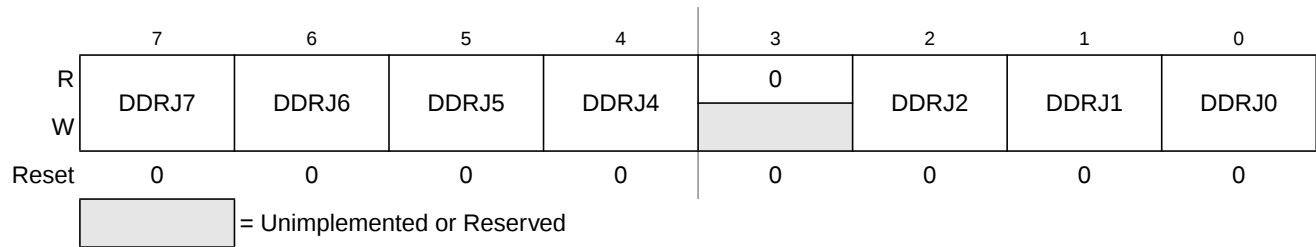
Figure 22-58. Port J Data Direction Register (DDRJ)
