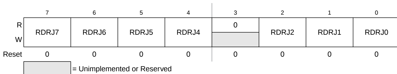
Figure 23-59. Port J Reduced Drive Register (RDRJ)
