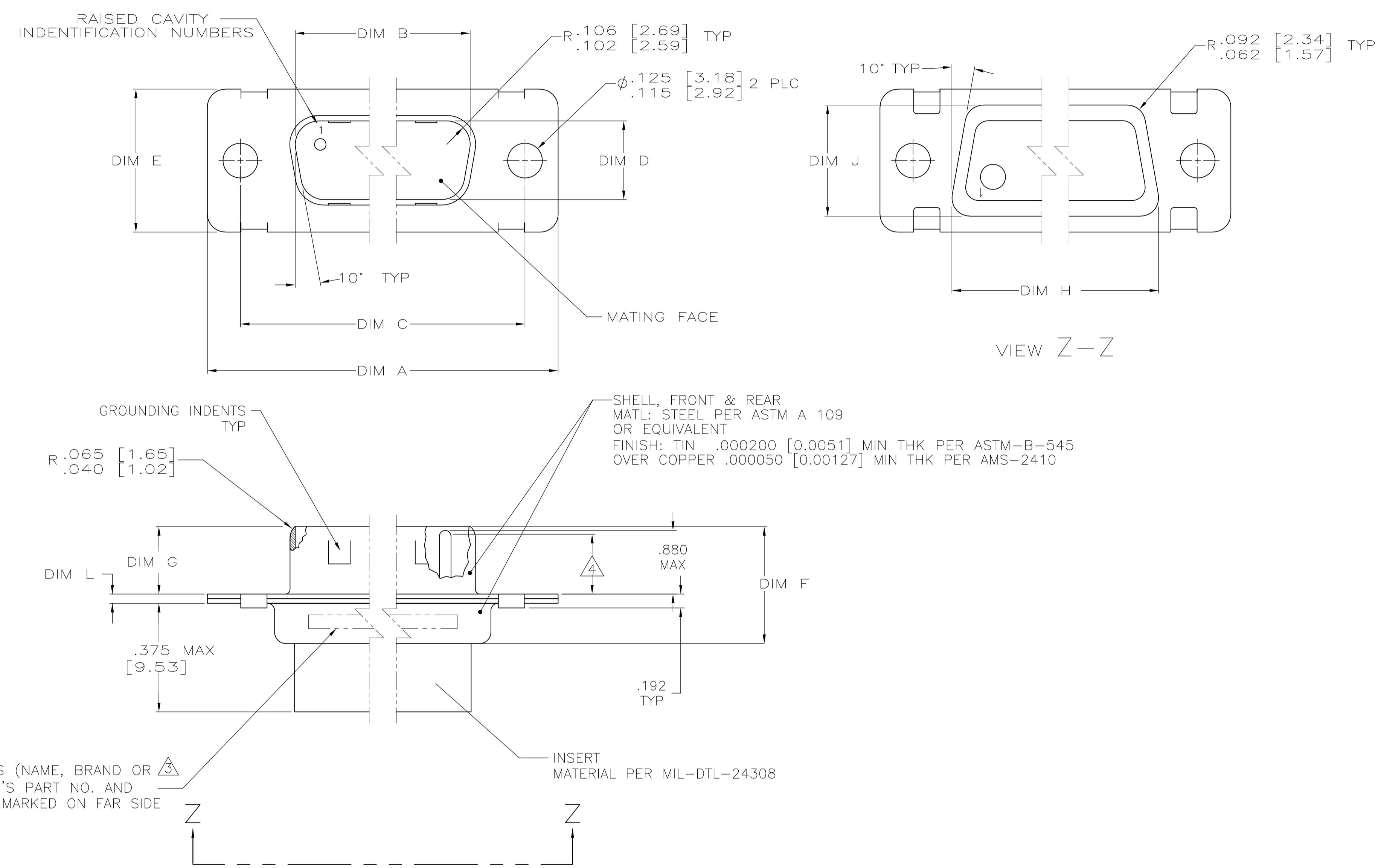
1. THIS CONNECTOR ASSEMBLY IS SUPPLIED WITH METAL CONTACT RETENTION CLIPS INSTALLED IN THE INSERT ASSEMBLY.
